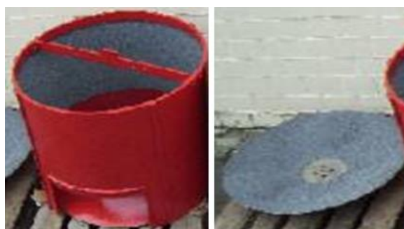
Fig.2. Drum and disc for potato peeler Source: own processing based on from Catalogue.
